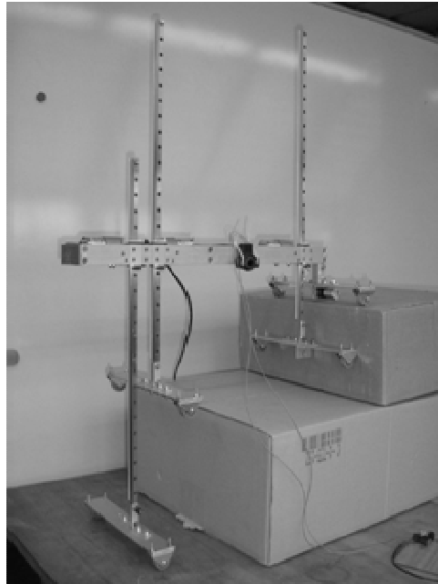
Fig. 10: Physical model of the stair-climbing module
